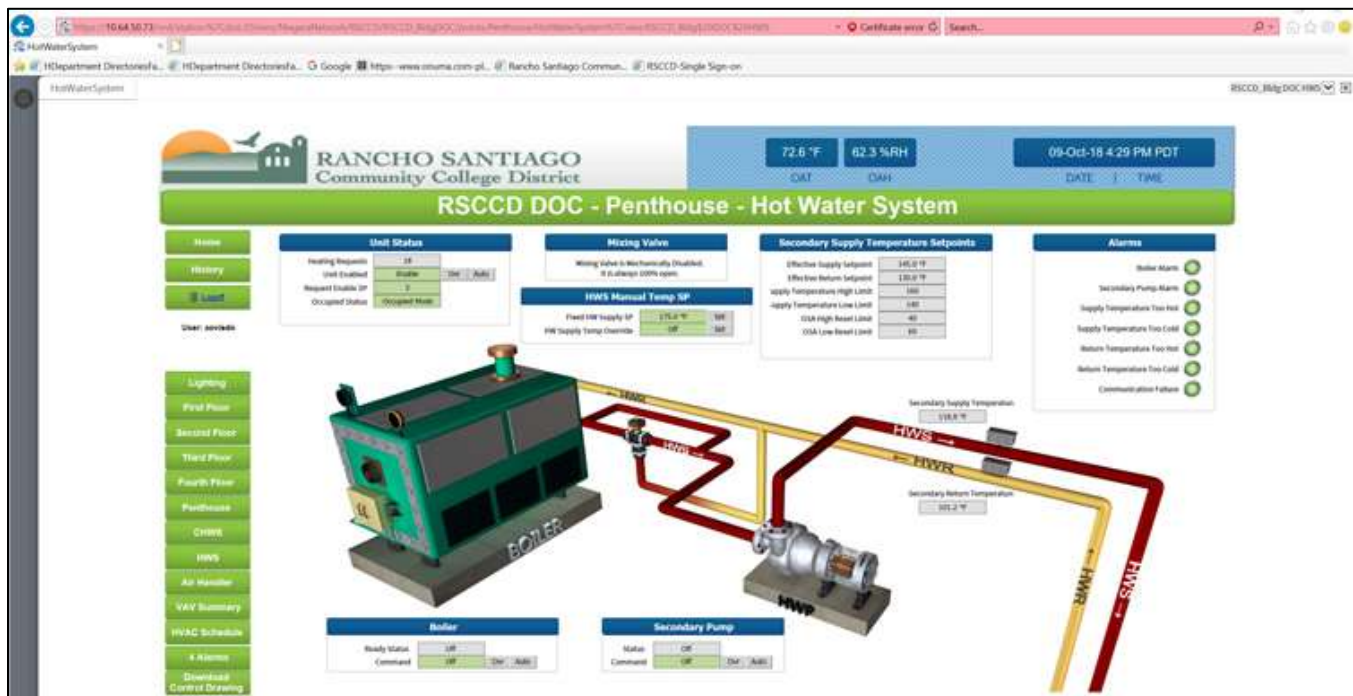
Figure 15. District Operation System EMS (view of Penthouse Hot Water System)
