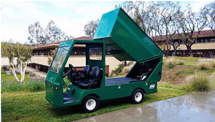
Figure 19. Burden cart with a hopper
