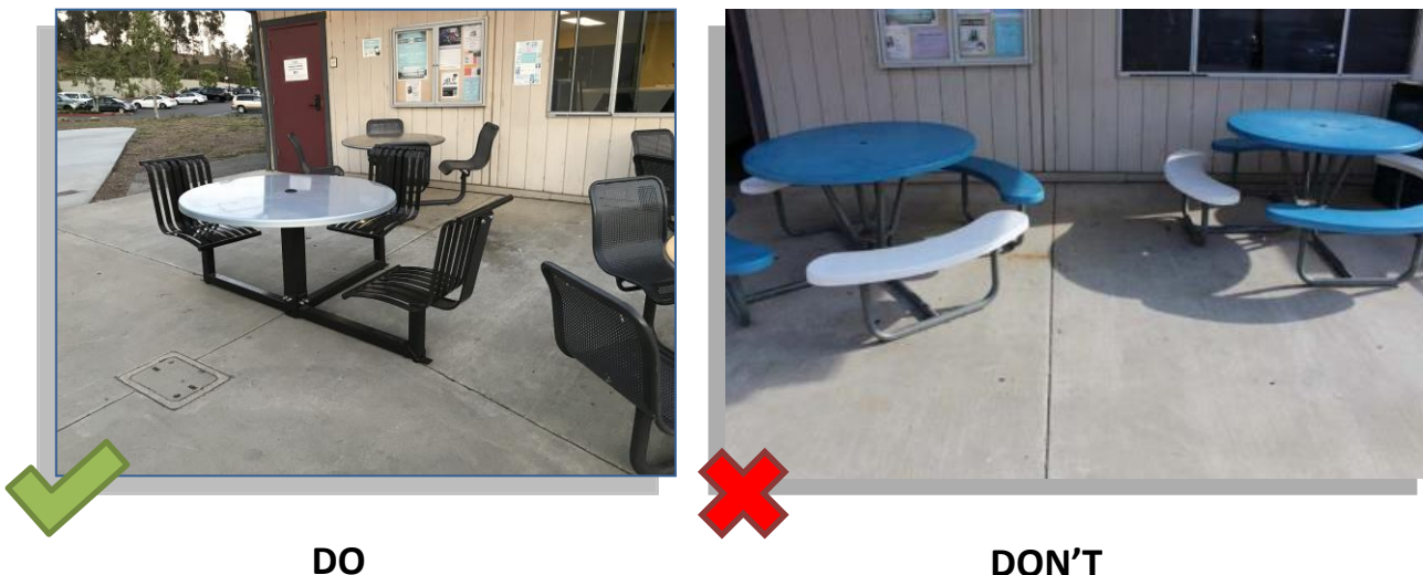
An accessible picnic table at left and non-compliant tables at right.
